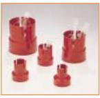
Side slots can be used as sight windows. Autoclavable at 121°C (250°F). 3 per package, 8 packages per case, except assortment.
